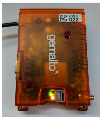
Figure 3: modem picture with status LEDs
