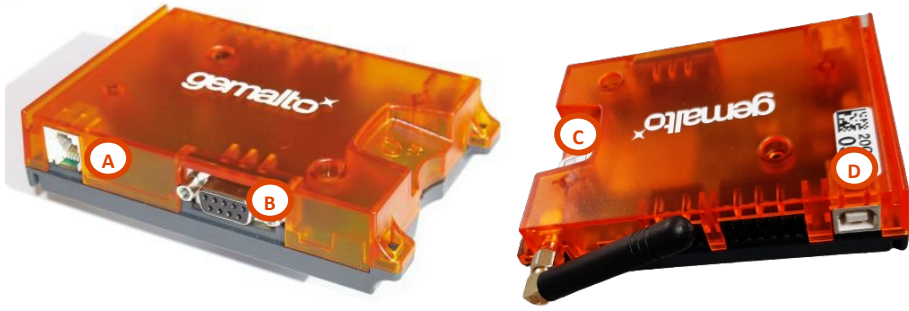
Figure 4: modem sockets and connectivity
