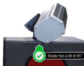
Figure 11: view from the front of the signal head: radar is leaning
