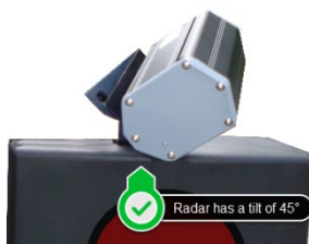
Figure 12: view from the front of the signal head: radar is leaning
