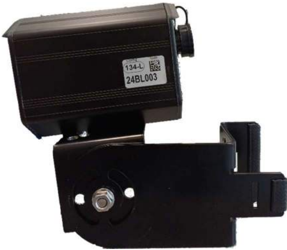
Figure 16 : distant detection installation < 5° vertical/0° horizontal
