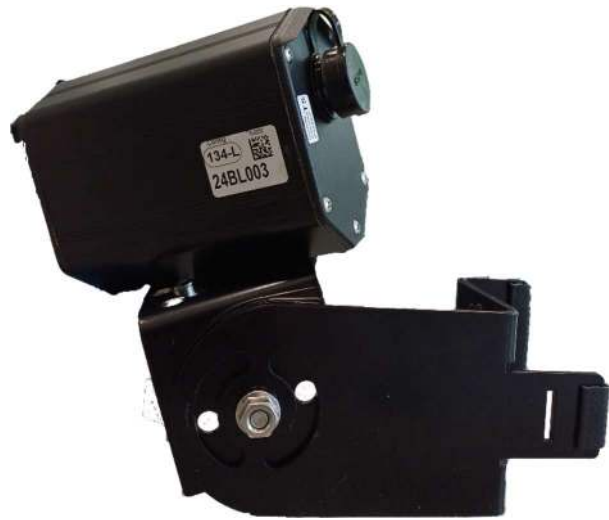
Figure 17 : installation for stop-line detection, radar on the right in the direction of travel 20° vertical/-30° horizontal
