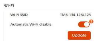
Figure 28: disable the Wi-Fi automatically after 60 minutes of inactivity
